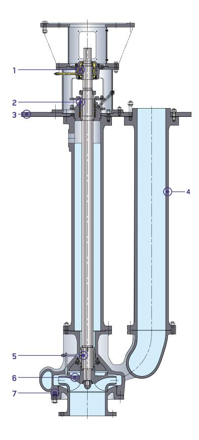
Stable shaft supported by greaselubricated angular contact ball bearings above the support flange and corrosion-resistant sleeve bearings with medium lubrication.
